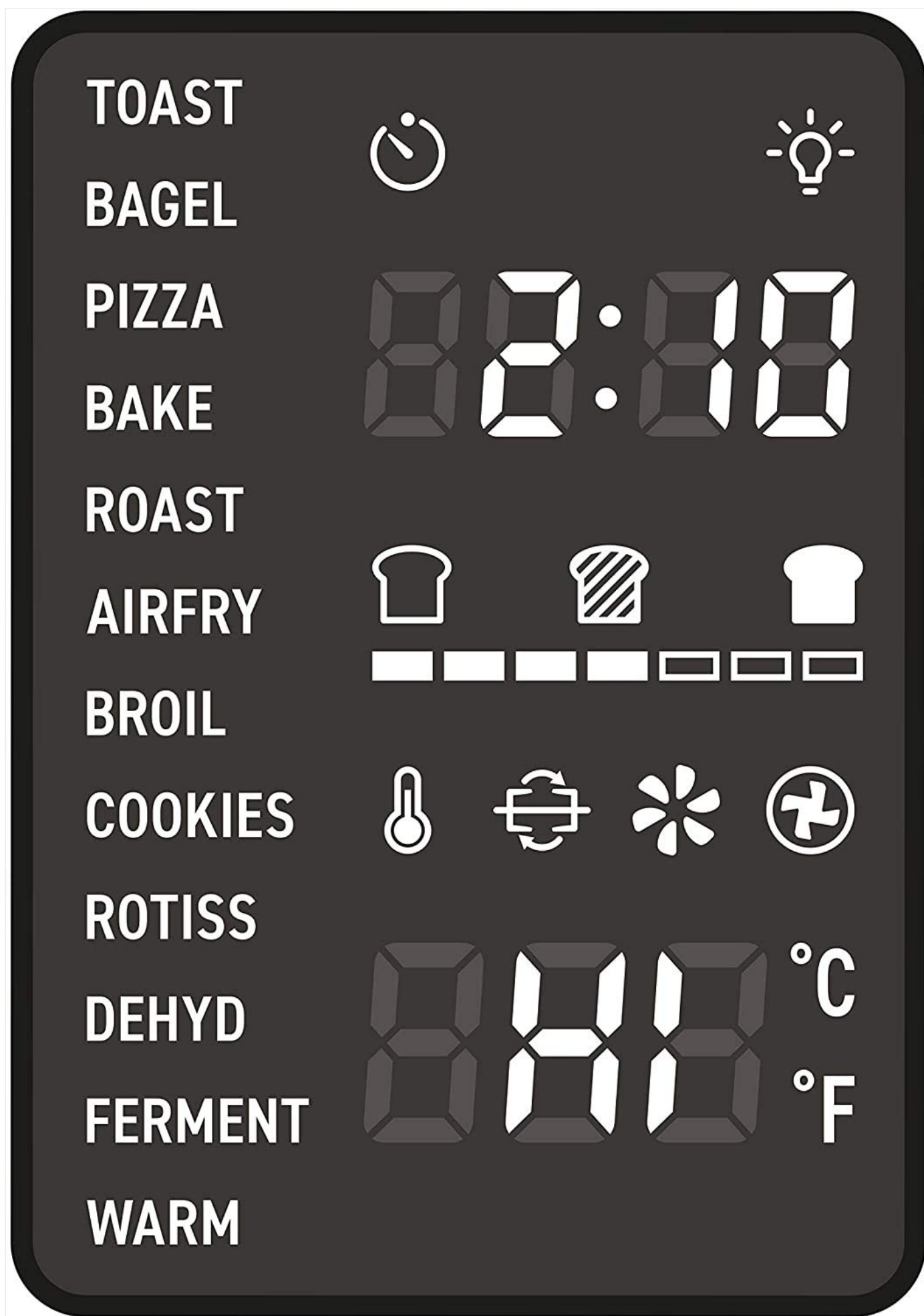
Image 3.2: Control Panel. This image shows a close-up of the digital control panel with various cooking presets like TOAST, BAGEL, PIZZA, BAKE, ROAST, AIRFRY, BROIL, COOKIES, ROTISS, DEHYD, FERMENT, and WARM, along
