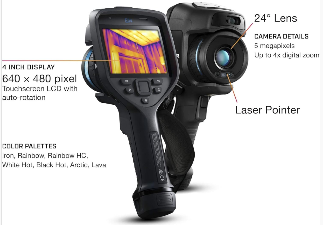
Figure 3: Display and lens features of the FLIR E54.
