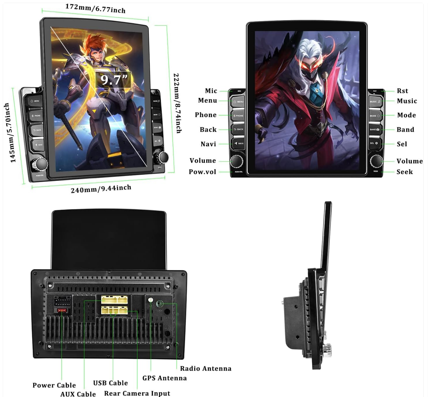
Figure 2: Product dimensions (Front, Side, Back views).
