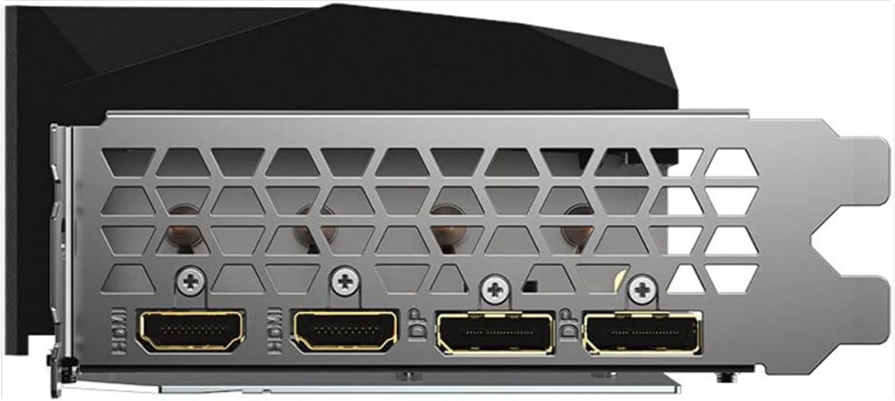
Figure 4: Rear panel with display output interfaces, including DisplayPort and HDMI ports.
