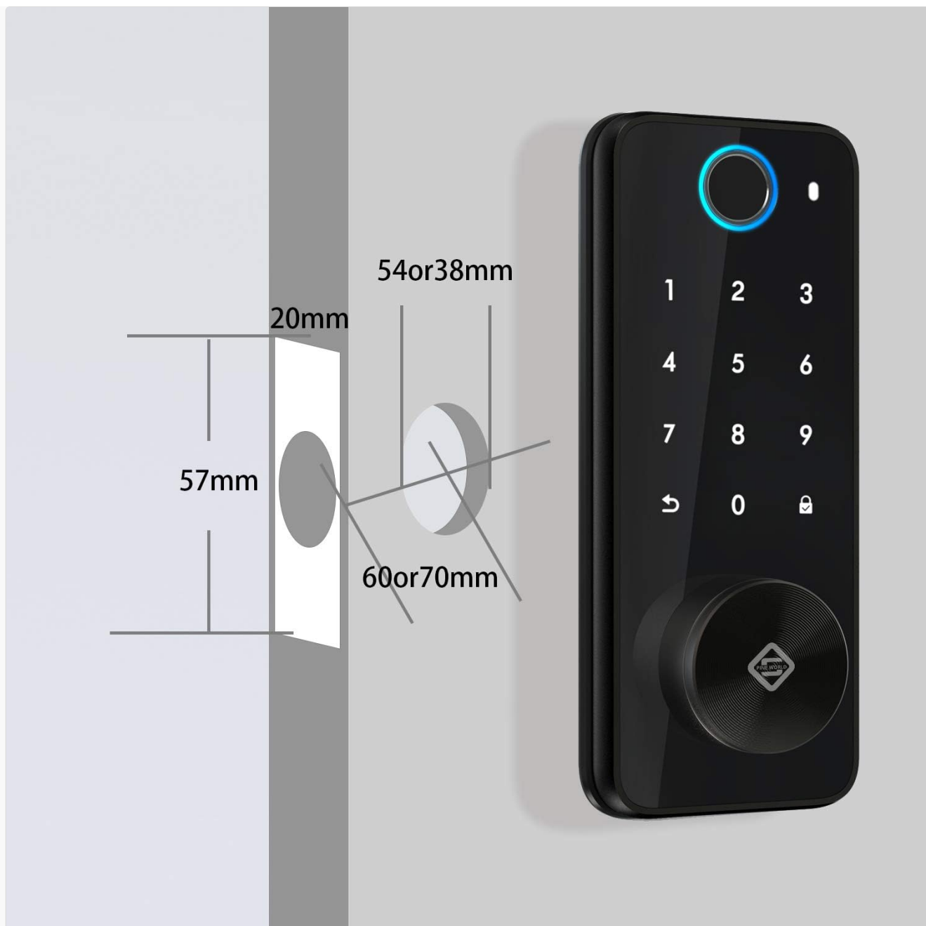
Image 3.1: Diagram illustrating the required door preparation dimensions for installation, including backset (60mm or 70mm) and bore hole diameters.
