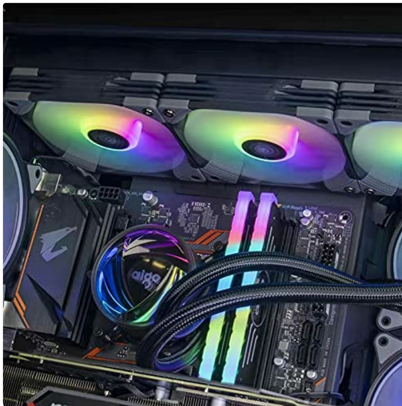
Image: The aigo AT240 liquid cooler installed within a PC case, showing the radiator mounted at the top and the CPU block connected to the motherboard, with ARGB lighting active.
