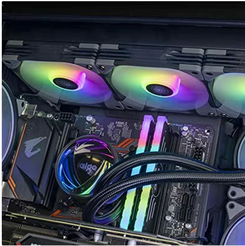
Image 3.1: The aigo AT360 liquid cooler fully installed within a computer case, demonstrating proper placement and cable management.
