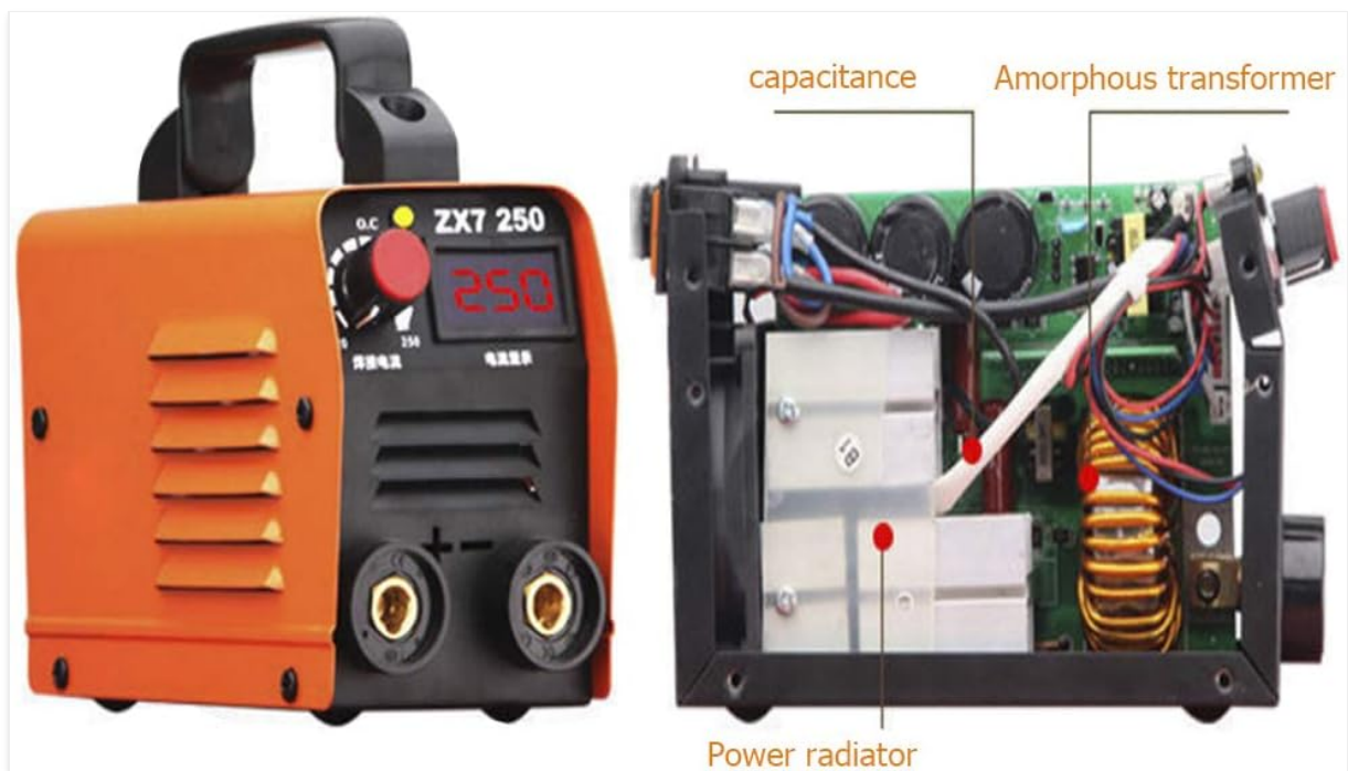
Figure 4.3: Internal view of the ZX7 250, highlighting key components such as capacitance, amorphous transformer, and power radiator.
