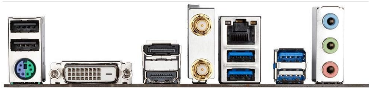
Figure 4.2: Rear I/O panel of the GIGABYTE A520M DS3H AC motherboard, featuring USB ports, HDMI, DVI-D, DisplayPort, LAN, Wi-Fi antenna connectors, and audio jacks.
