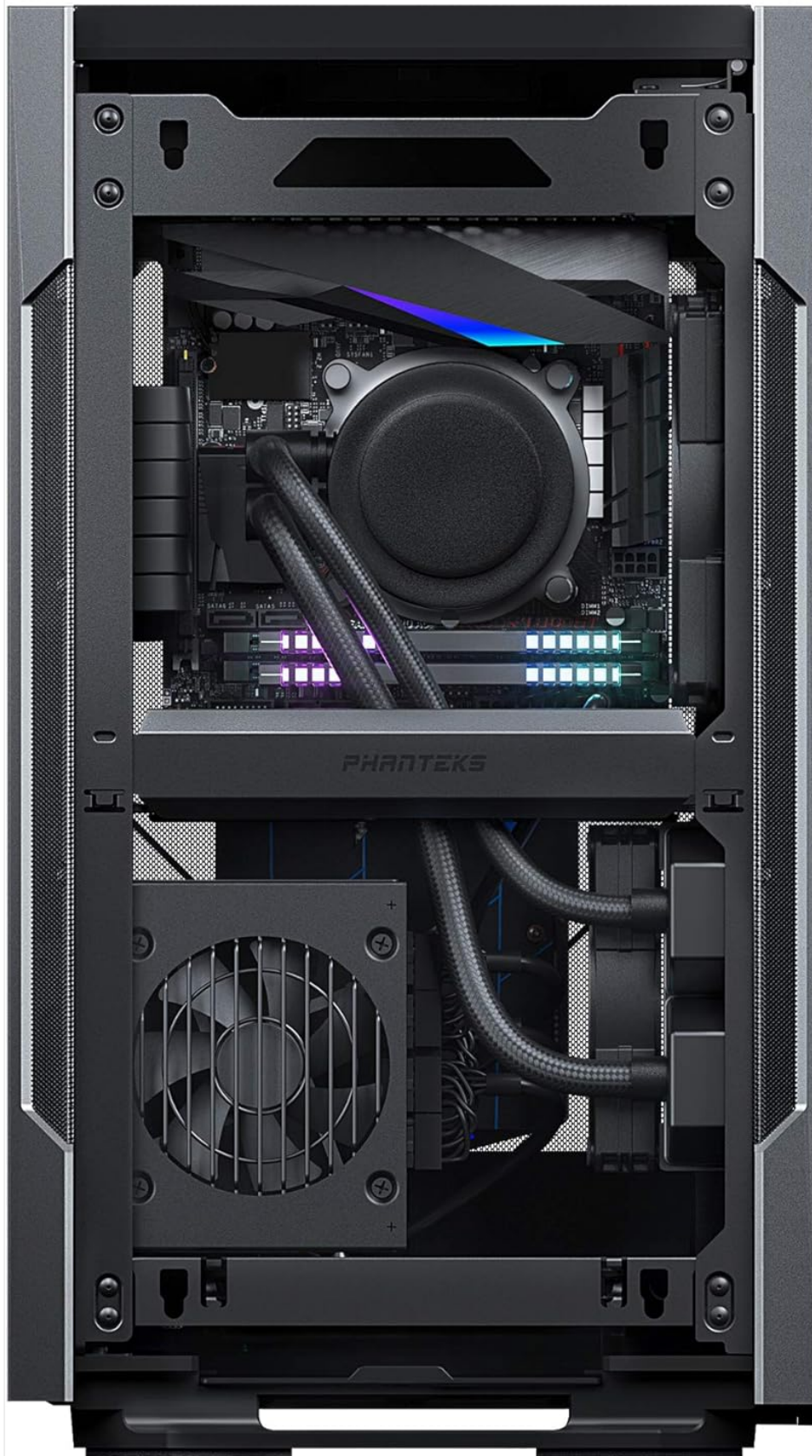
Figure 4.3: Internal layout with a motherboard, CPU cooler, and vertically mounted graphics card.
