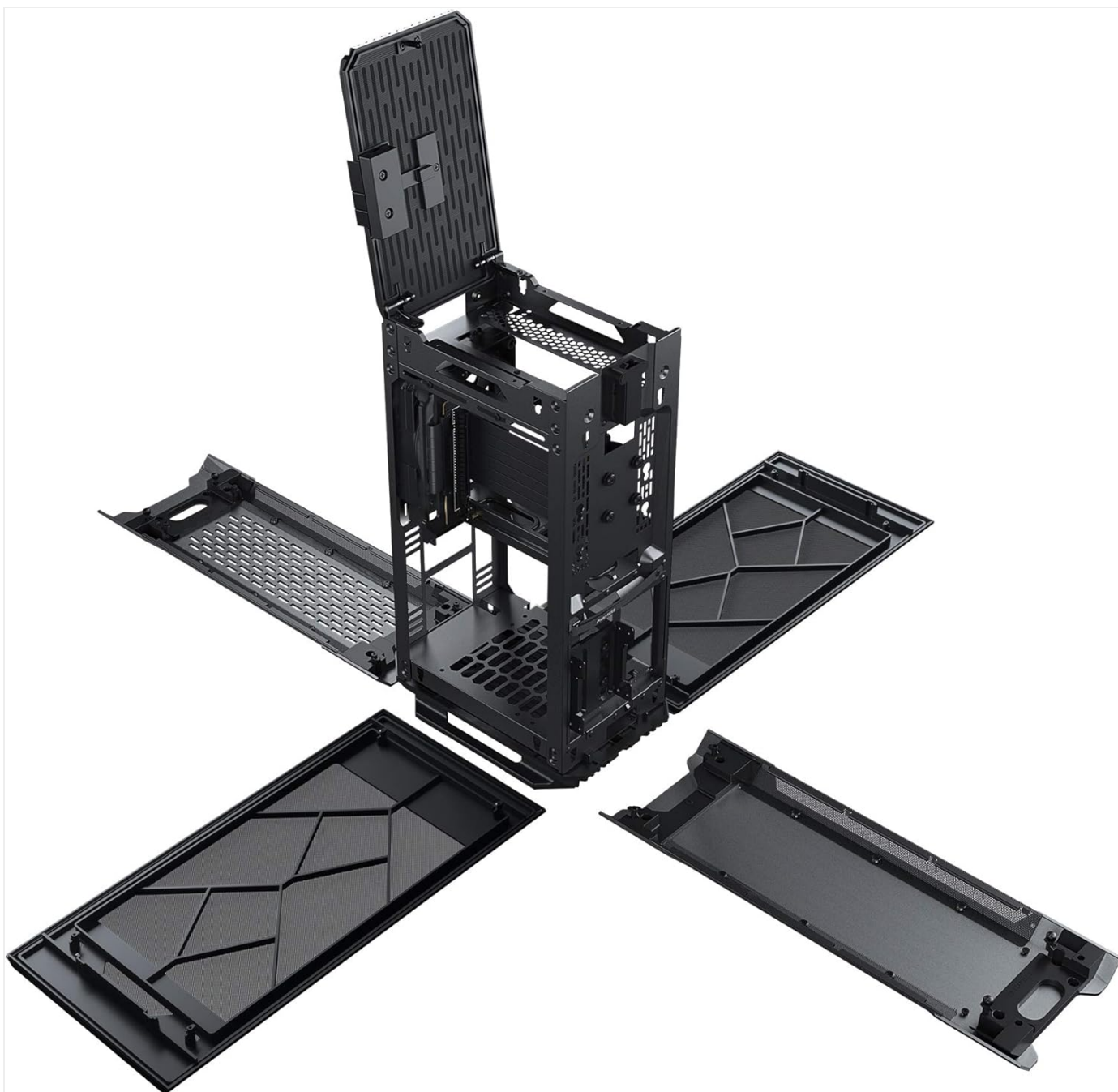
Figure 4.1: Exploded view of the Evolv Shift 2 Air, showing removable panels and internal frame.
