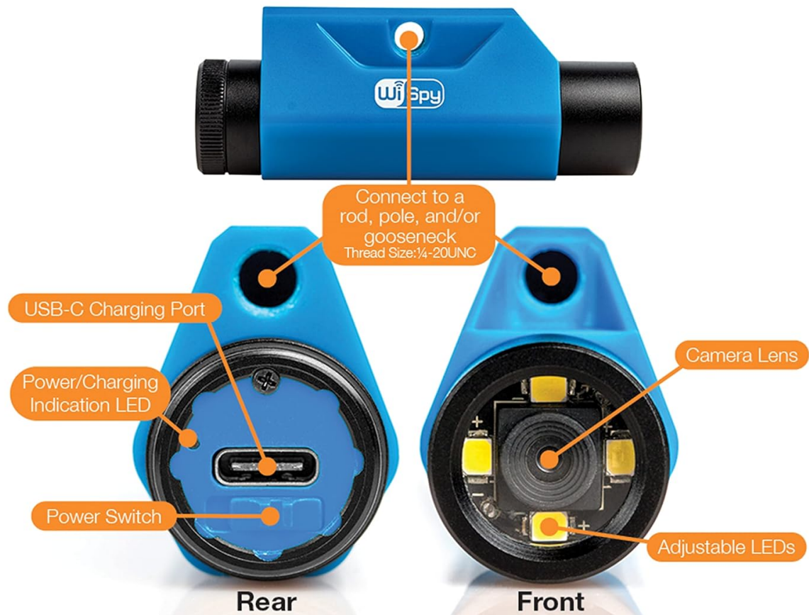
Image: Detailed view of the Wispy CF-200 camera, showing the USB-C charging port, power switch, camera lens, and adjustable LEDs.
