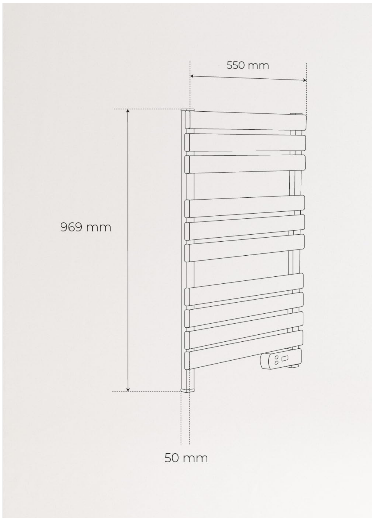
Figure 5.2: Dimensional drawing showing the height (969 mm), width (550 mm), and depth (50 mm) of the unit.
