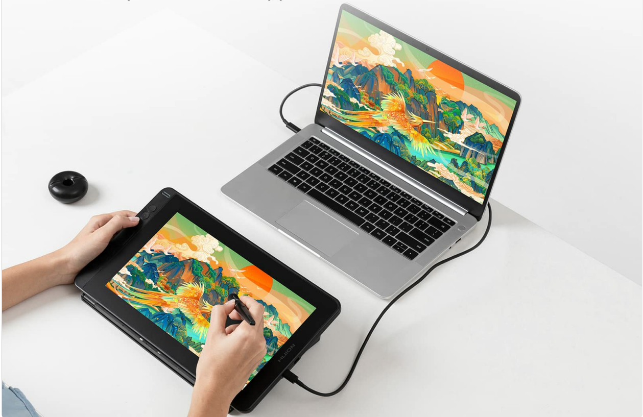
Image 3: Connecting the KAMVAS 12 to a laptop using a USB-C to USB-C cable.
