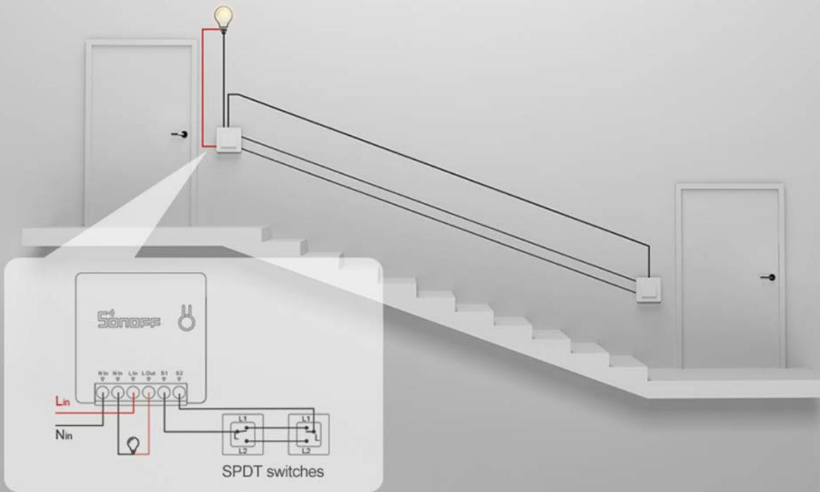
\*External switches are not limited to two-way control switches.
