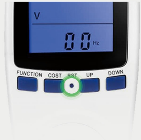
Figure 4.1: Steps to set the electricity cost per kWh on the monitor.
