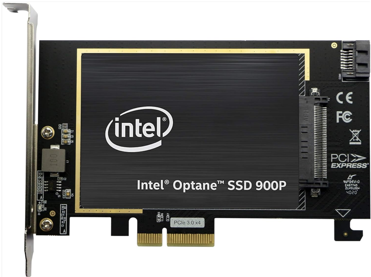
Image: A detailed view of the expansion card, highlighting its SATA 7PIN interface, PCI-E 3.0 x4 interface, and U.2 (SFF-8639) connector.
