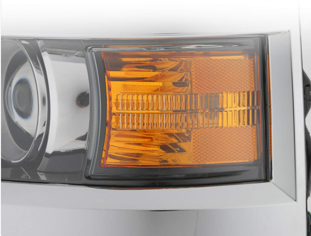
Image 6.1: Micro-Prism Reflectors for Enhanced Light Distribution
