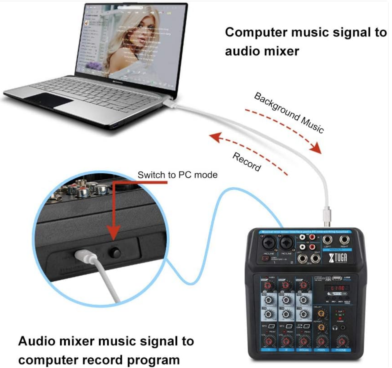
Diagram illustrating how to connect the XTUGA AM6 mixer to a computer via USB for recording audio from the mixer to the computer and playing background music from the computer through the mixer.
