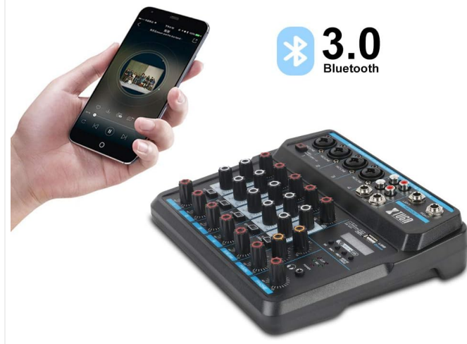
Figure 6: Connecting a mobile phone via Bluetooth to the XTUGA AM6 mixer.
