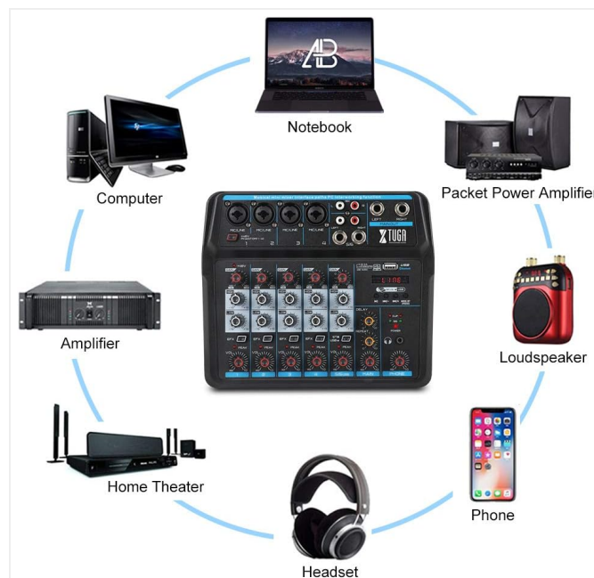
Figure 7: Connecting the mixer to a computer for sound card functionality.
