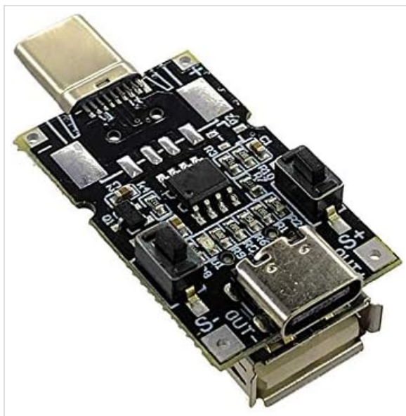
Image 1: Top-down view of the JacobsParts USB C QC Voltage Trigger Decoy Module, showing the USB-C male connector, control buttons, and various electronic components on the circuit board.
