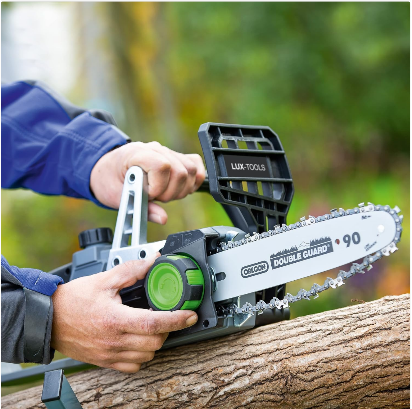
Image 4.1: A user demonstrating the adjustment of chain tension using the integrated knob.
