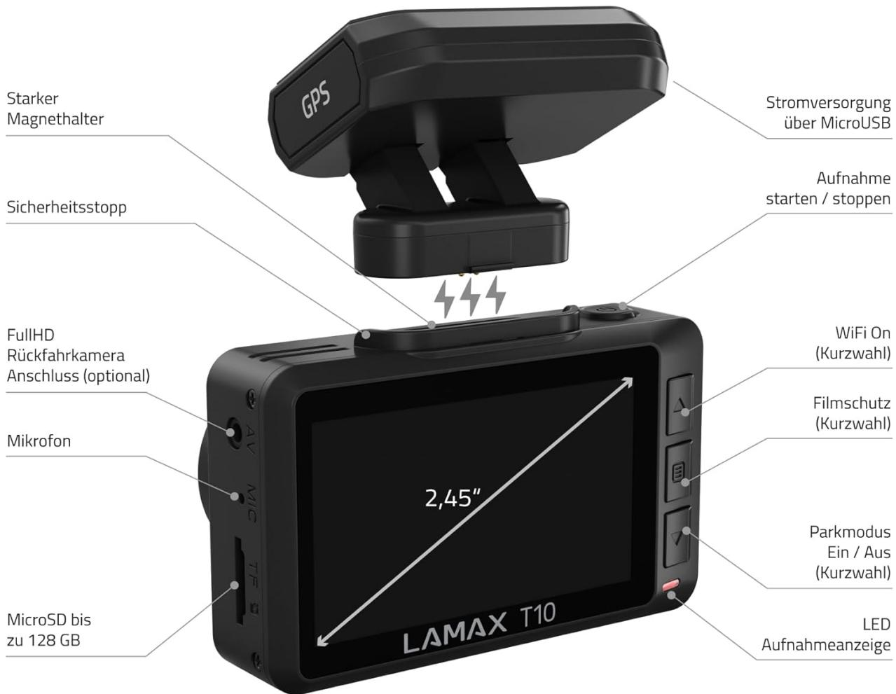
Detailed diagram showing the various ports, buttons, and indicators on the LAMAX T10 Dashcam, including the magnetic power connection, USB port, control buttons, microphone, and microSD card slot.
