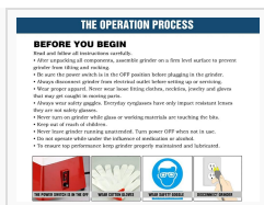
Image 2.1: A collage of safety reminders, including ensuring the power switch is off, wearing protective gloves and safety goggles, and disconnecting the grinder from the power outlet.
