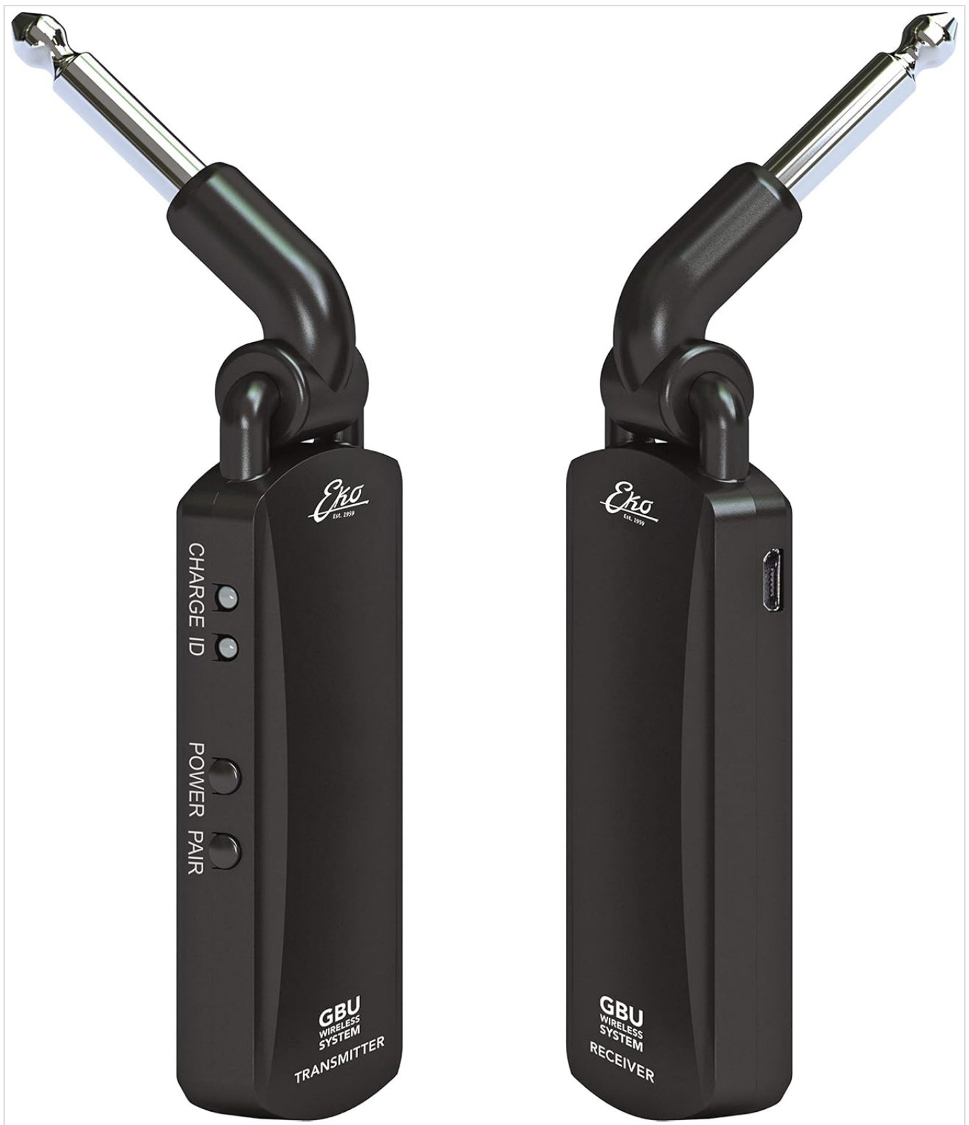
Figure 2.2: Eko GBU Wireless System units demonstrating adjustable jacks.
