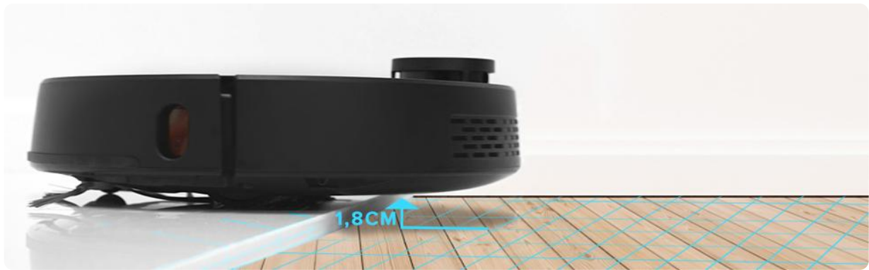
Image 9.1: The robot's ability to climb obstacles up to 1.8 cm.
