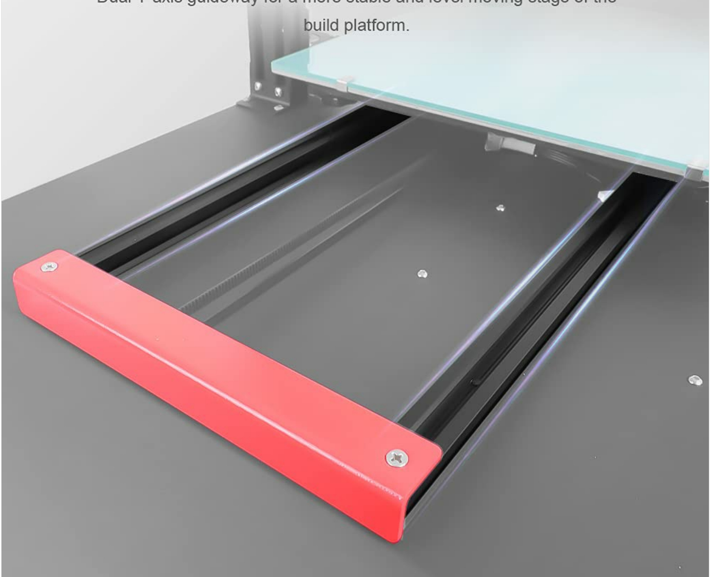
Figure 4.2: Dual Y-axis guideway for stable build platform.
