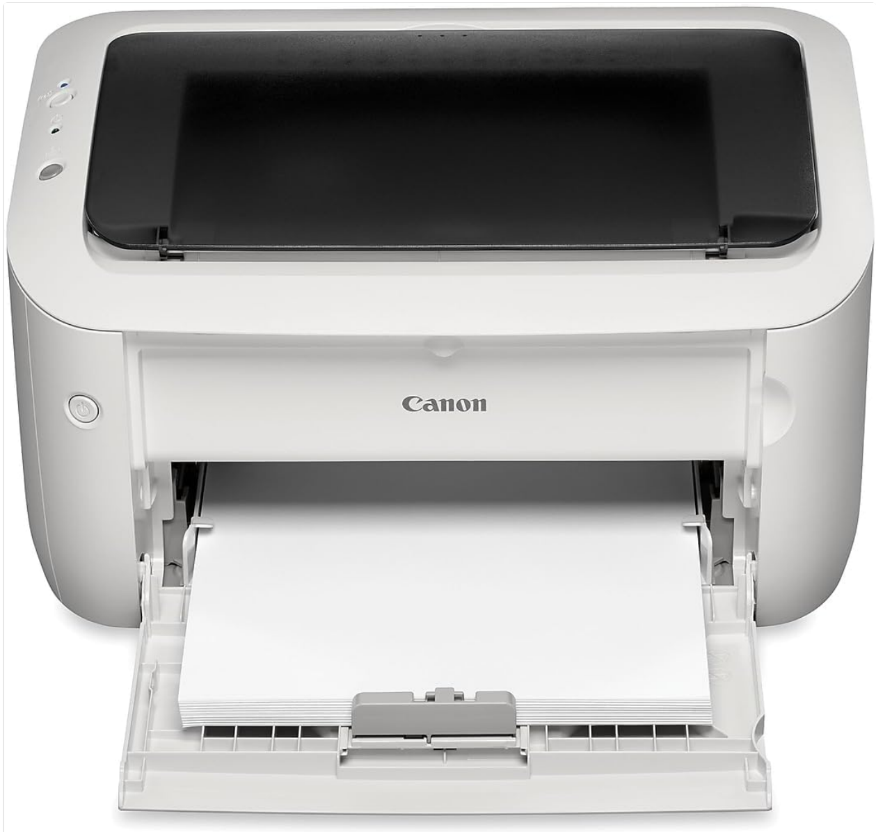
Figure 4.2: Loading Paper. This image shows the front paper tray pulled out with a stack of paper loaded, demonstrating the paper loading process.
