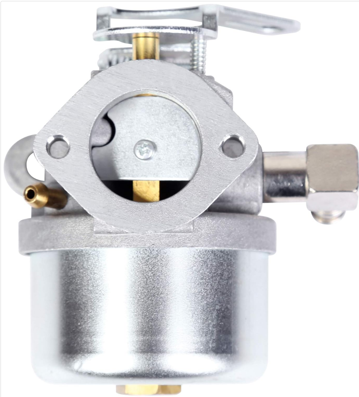
Image 3: Front view of the carburetor, showing the intake port.
