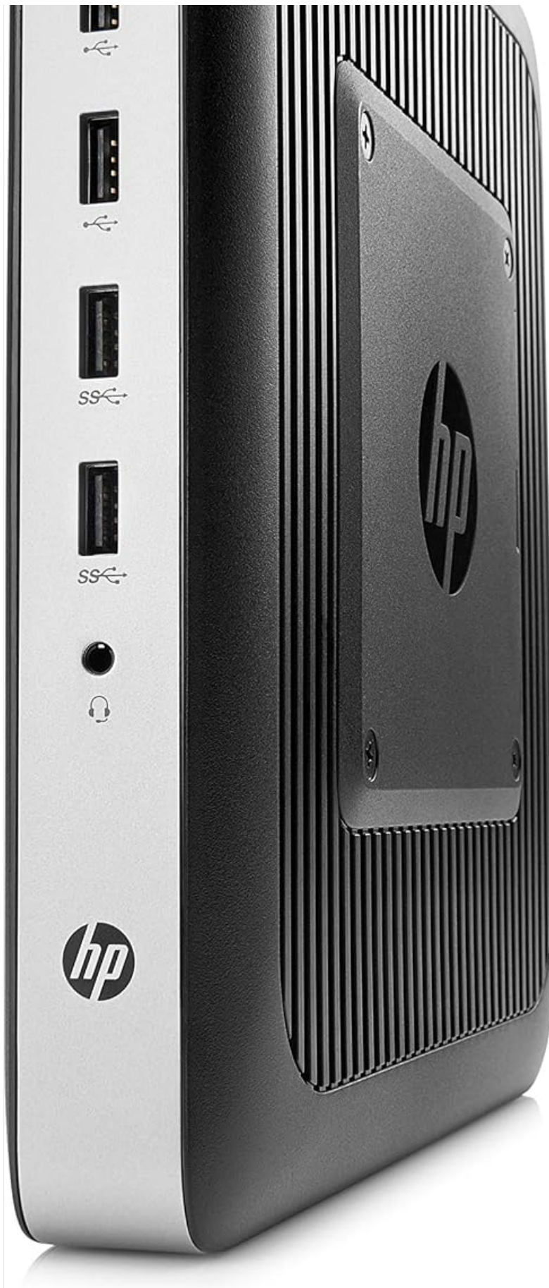
Figure 1: Front and side view of the HP t630 Thin Client. This image highlights the front panel with two SuperSpeed USB 3.0 ports, two Hi-Speed USB 2.0 ports, a headset jack, and the power button. The side panel features ventilation grilles and a mounting bracket.
