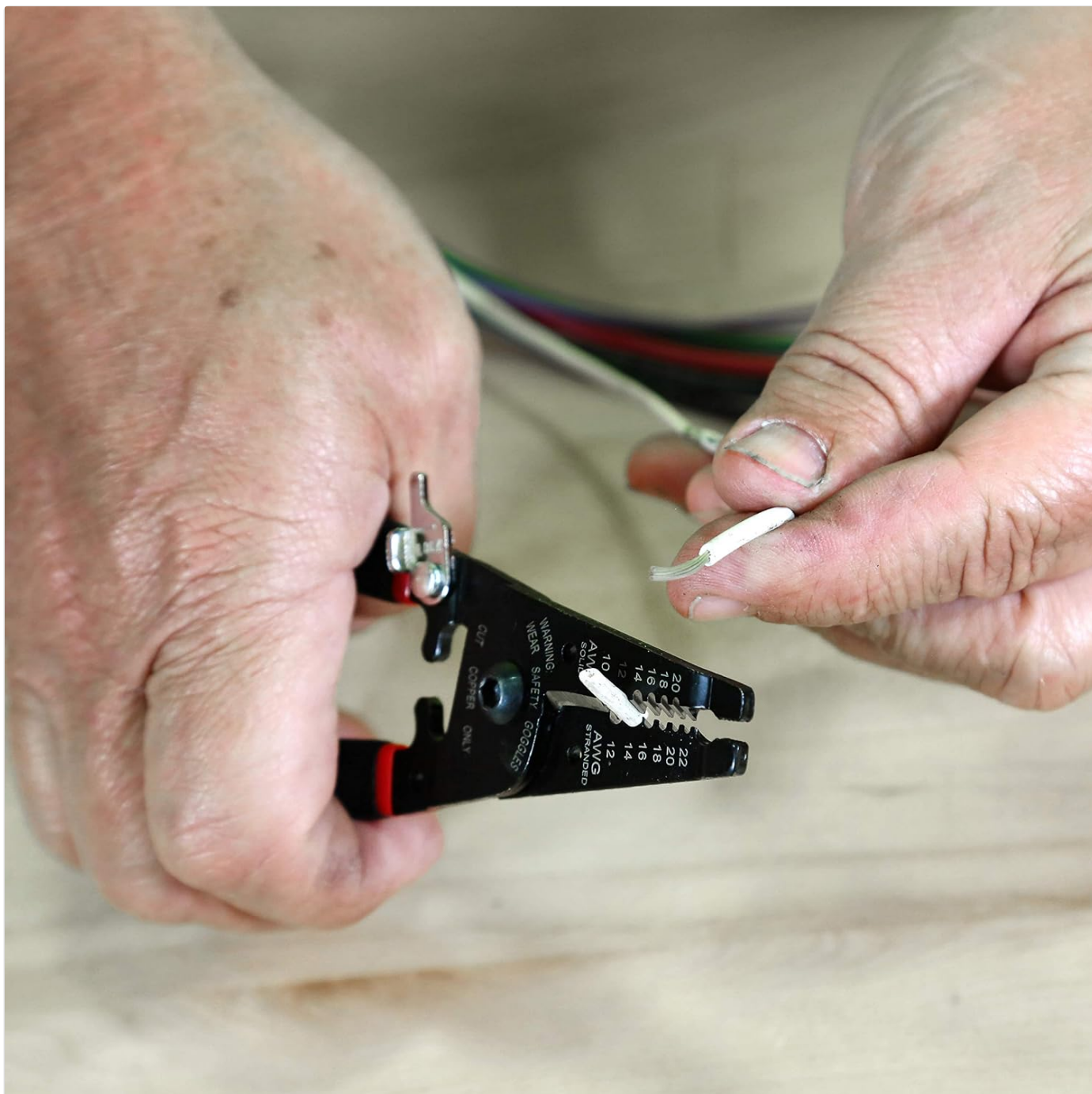
Image: The stripped insulation being removed from the wire.
