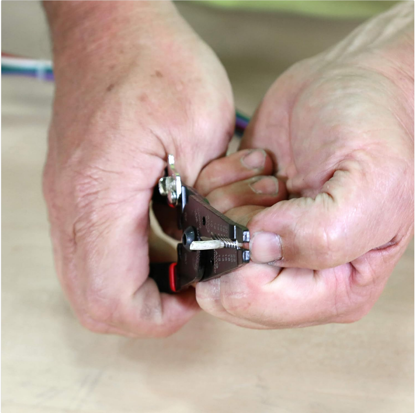
Image: Demonstrating the wire stripping process. The wire is inserted into the correct gauge slot.
