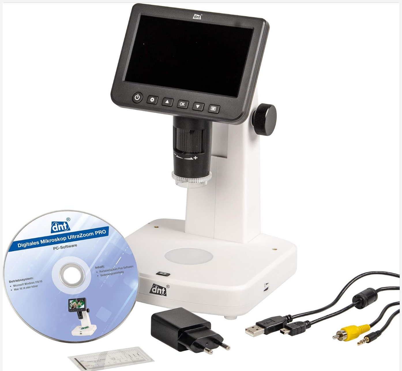
Image 2.1: Overview of the dnt UltraZoom PRO Digital Microscope and its complete set of accessories.
