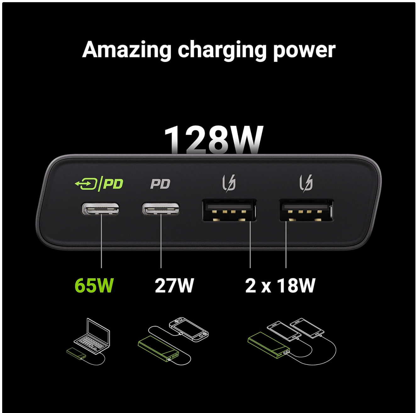
Image 4.1: Overview of the Green Cell PowerPlay Ultra ports, showing two USB-C Power Delivery ports (65W and 27W) and two USB-A ports (2 x 18W), totaling 128W output.
