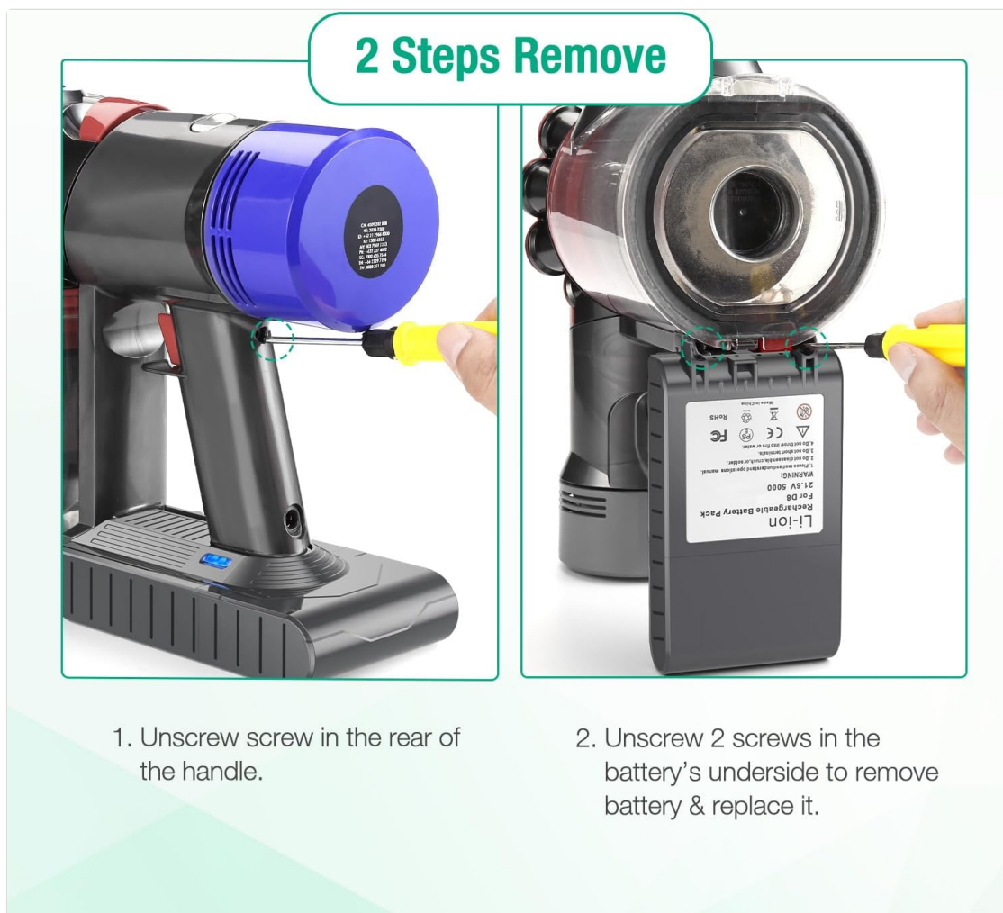
Figure 4: Step-by-step guide for battery replacement.
