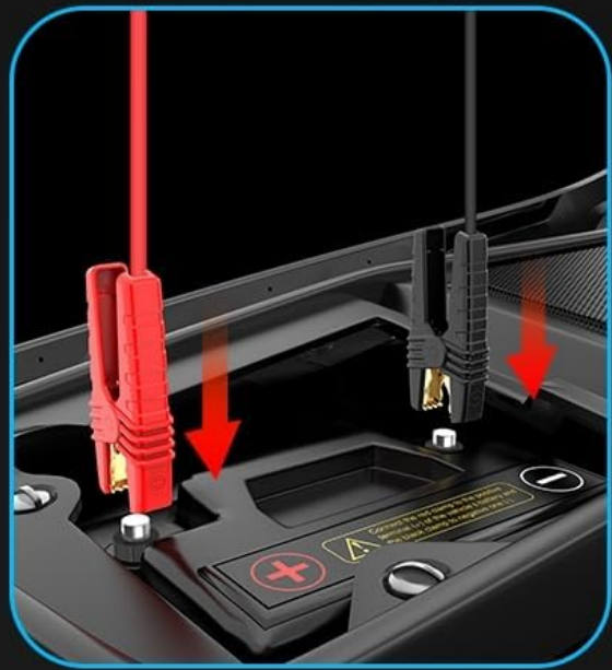
② Connect with the battery terminal, red "+" black "-"
