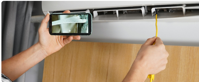
Using the endoscope for HVAC system inspection.
