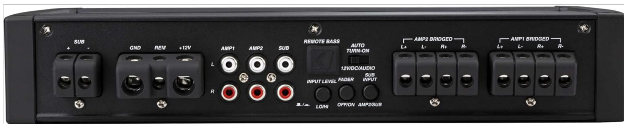
Figure 2: Rear panel connections for power, ground, remote, input, and speaker outputs.
