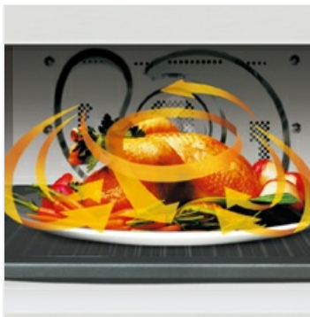
Figure 4.2: Illustration showing the hot air circulation during convection cooking for even heat distribution.
