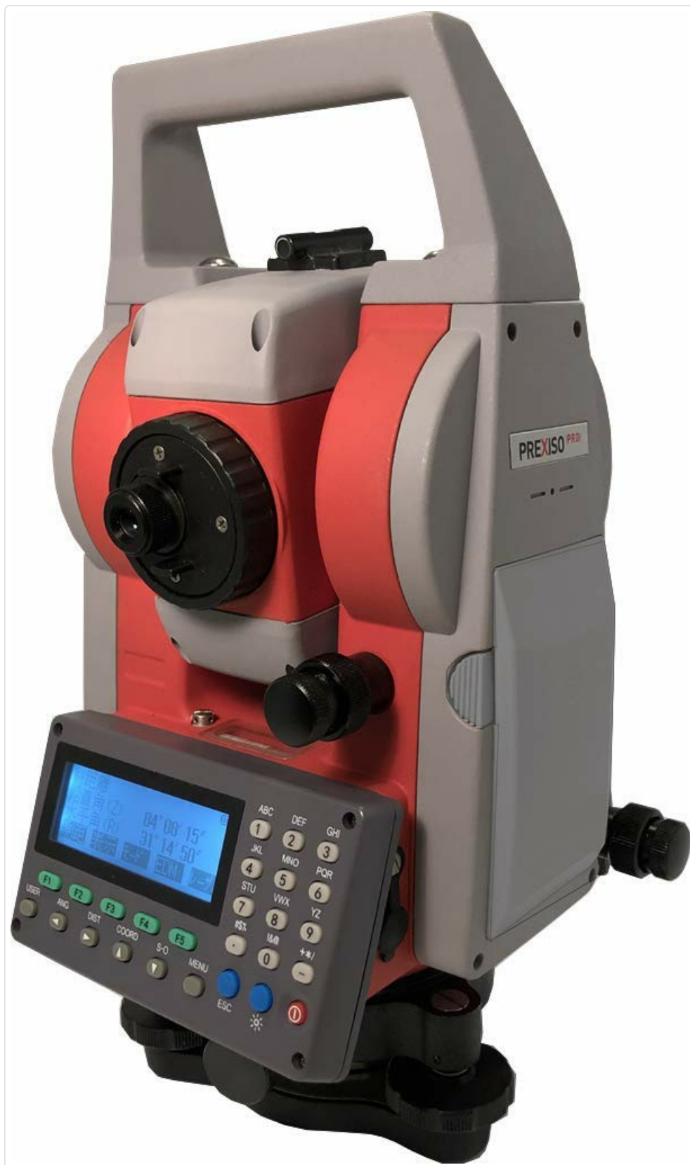
Figure 5.2: Non-Prism Measurement. The MT-105 can measure distances from a minimum of 1.6m (0.5m in non-prism mode), making it suitable for narrow spaces. It includes a laser pointer for targeting.
