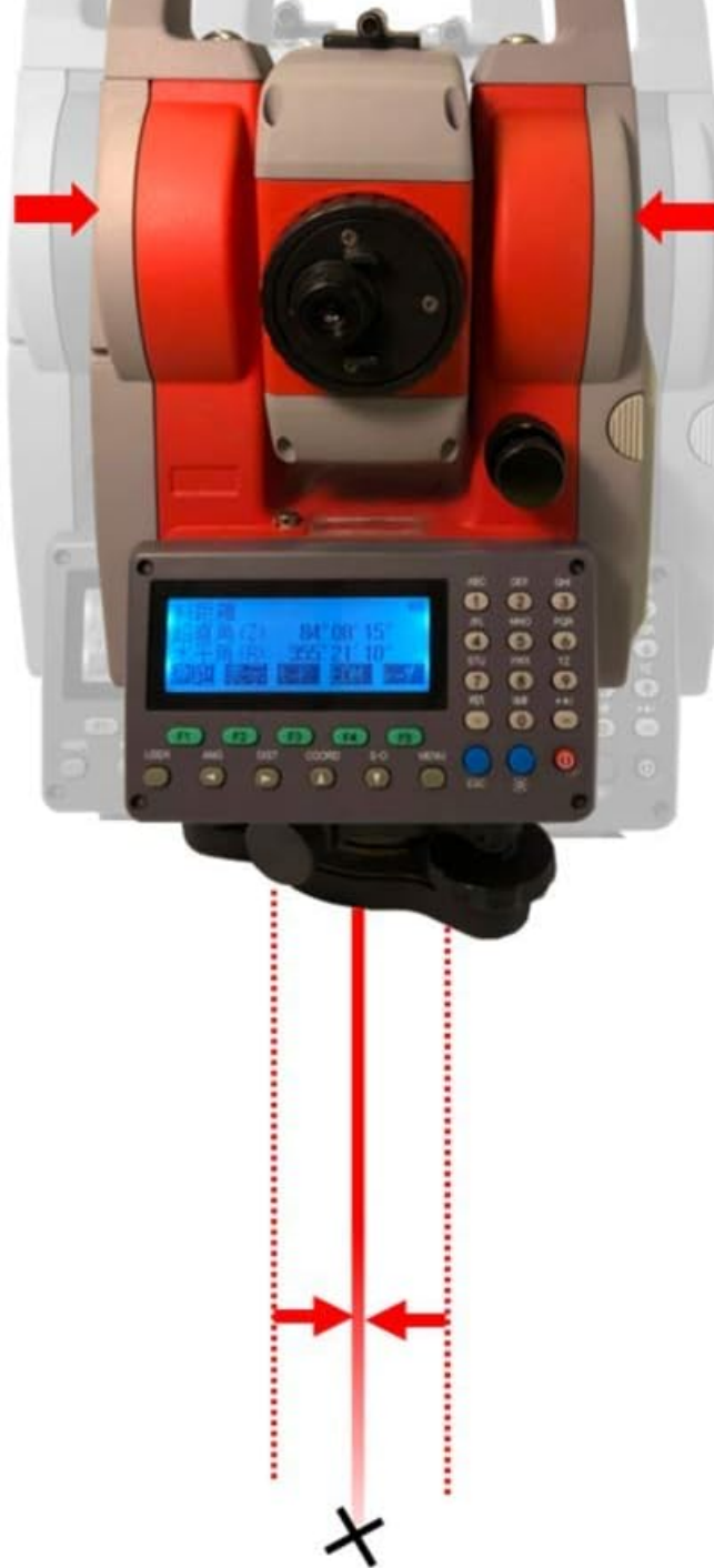
Figure 4.2: Laser Plummet and Shifting Function. This image demonstrates how the laser plummet and shifting mechanism simplify centering the instrument over a point.
