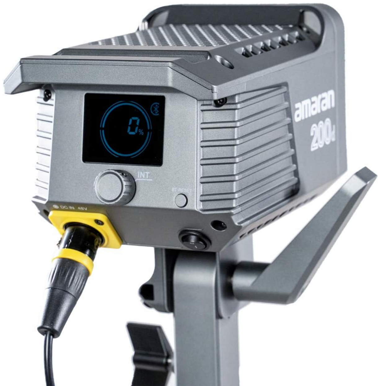
Figure 5.1: The control panel of the Amaran 200d, showing the display and adjustment knob.
