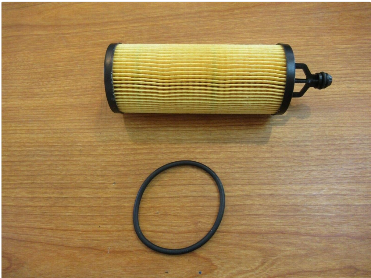
Figure 5: Mopar oil filter element with a new O-ring, ready for installation.
