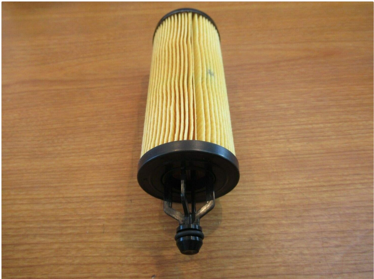
Figure 6: End view of the Mopar oil filter element, showing its pleated design and internal structure.
