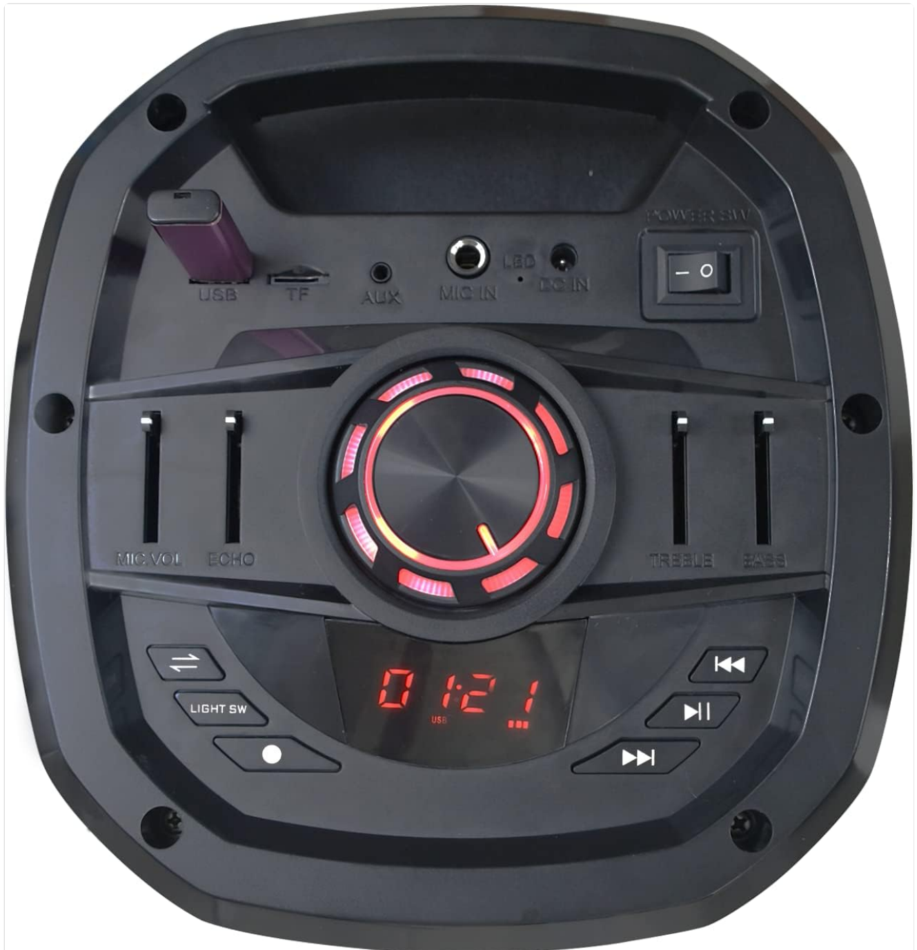
Figure 2: Top control panel of the PSL300B, featuring USB and TF card slots, AUX input, MIC IN, DC IN, power switch, master volume knob, microphone volume, echo, treble, bass sliders, light switch, and playback controls.
