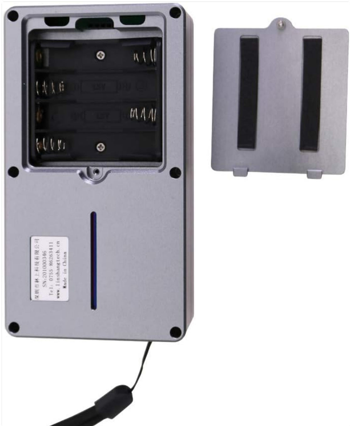
Figure 4.1: Rear view of the LS201 meter with the battery cover removed, revealing the battery slots for installation.
