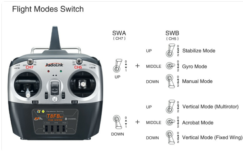
Figure 5: Detailed diagram showing how to configure CH5 and CH7 switches on a Radiolink transmitter to select different flight modes (Stabilize, Gyro, Manual, Vertical Multirotor, Acrobat, Vertical Fixed Wing).
