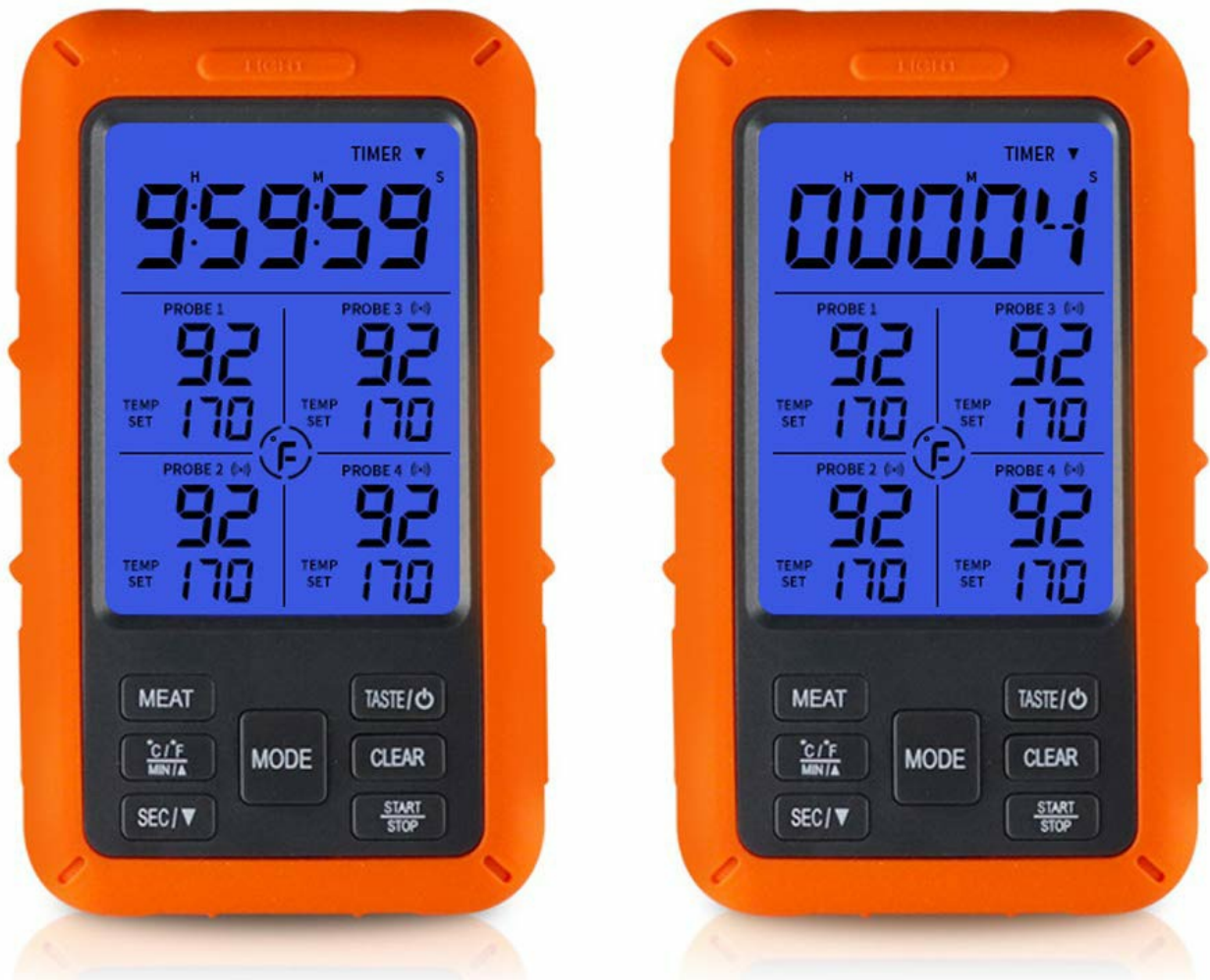
Image 5.3: The main unit display demonstrating the timing and countdown functions, showing a set countdown time and a count-up timer.
