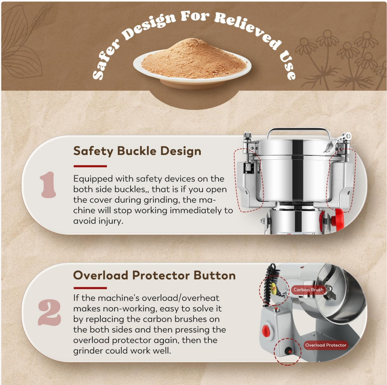
Image 2: Illustration of the safety buckle design, which stops the machine if the cover is opened, and the overload protector button, used for resetting after carbon brush replacement.
