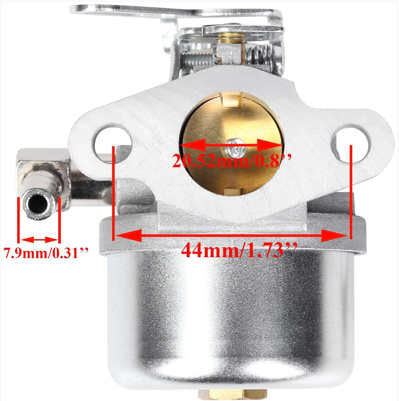
Image 5.3: Frontal dimension measurements of the carburetor, indicating key distances for fitment verification.
