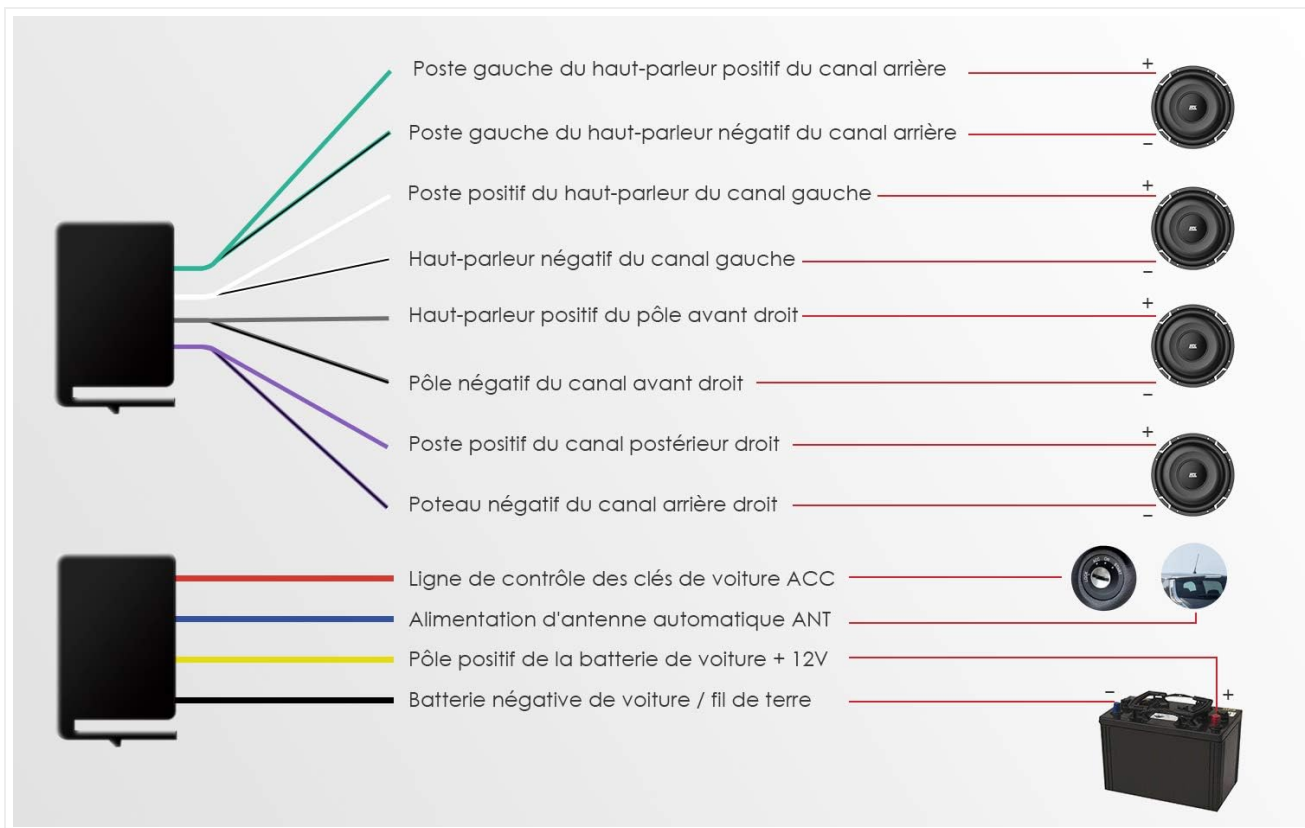
Figure 3.2: Detailed wiring diagram for the ieGeek K305.
