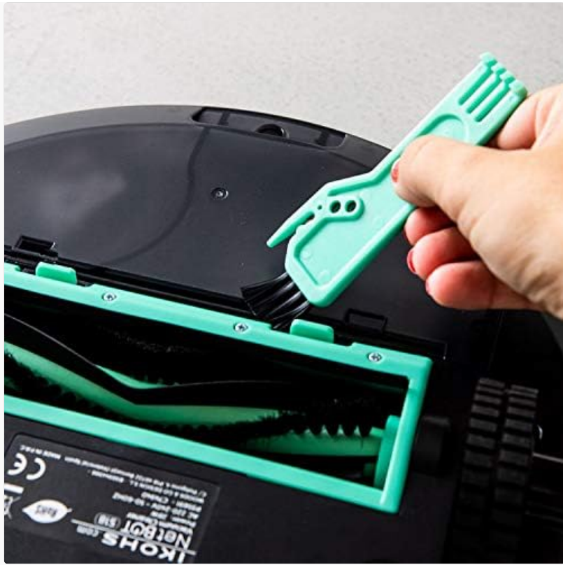
Figure 6.1: Using the cleaning tool to remove hair and debris from the main rolling brush.
