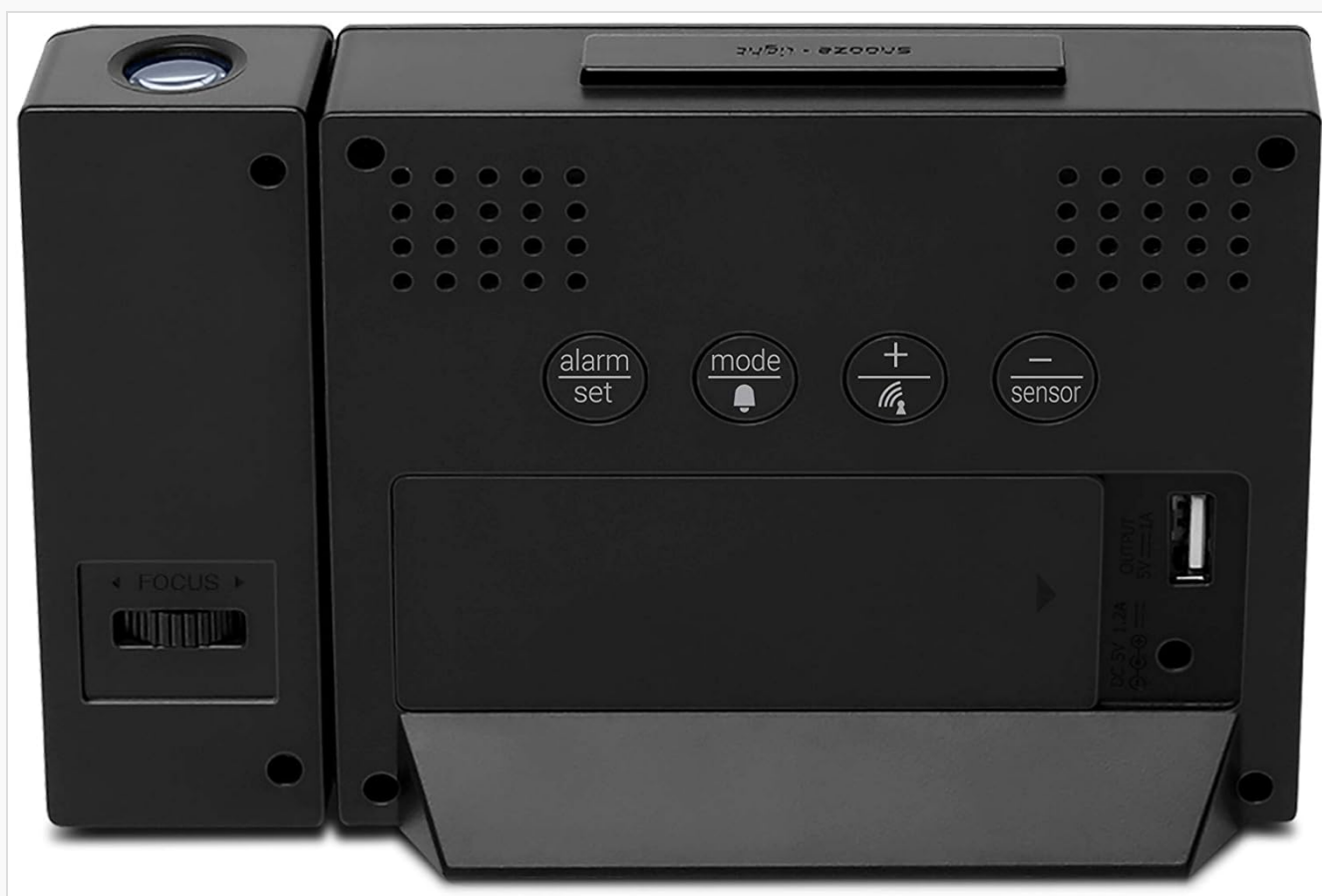
Figure 4.2: Rear panel of the clock, featuring buttons for 'alarm set', 'mode', '+', '-', 'sensor', and a USB charging port. The projection lens is visible on the left side.
