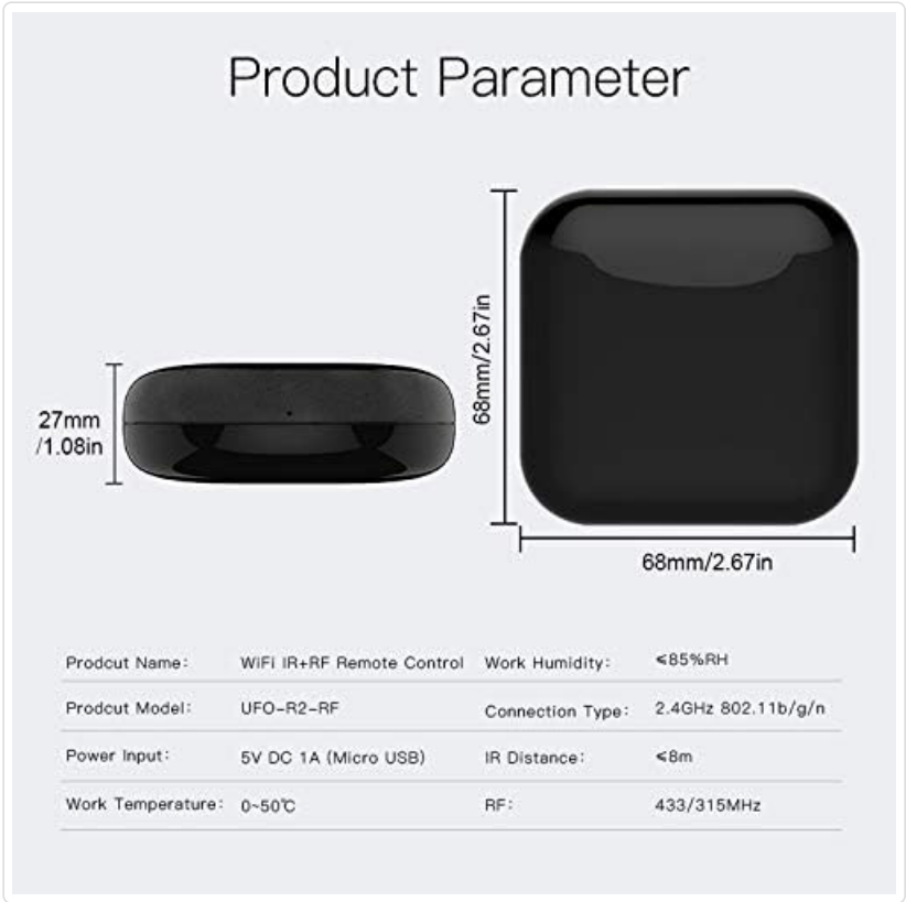
Figure 3.2: Diagram illustrating the physical dimensions of the MoesGo Universal Remote Controller (68mm x 68mm x 27mm) and basic product parameters.
